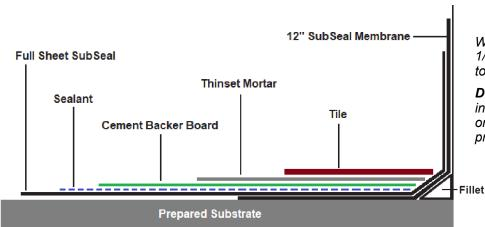
When using a sealant, apply a 1/4" bead of sealant every 8" to the SubSeal membrane.
